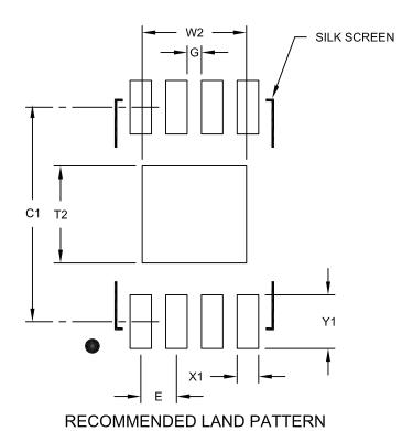
Units **MILLIMETERS Dimension Limits** MIN MOM MAX Contact Pitch Ε 0.50 BSC Optional Center Pad Width W2 1.46 Optional Center Pad Length T2 1.36 Contact Pad Spacing C1 3.00 Contact Pad Width (X8) X1 0.30 Contact Pad Length (X8) <u>Y1</u> 0.75 Distance Between Pads G 0.20
