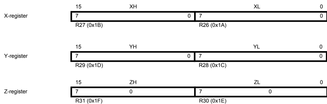
Figure 6-3. The X-, Y-, and Z-registers
